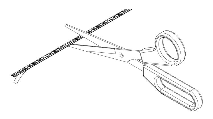
The LED strip can be separated or shortened every 33.3 mm. On the back of the LED strip is a double-sided heat-conducting adhesive tape, which allows installation of the LED strip. Professional LED strips can be cut with scissors.
