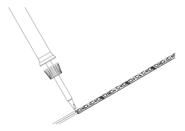
The Professional LED Strips are connected via a lead connection to the connection pads provided for this purpose.
